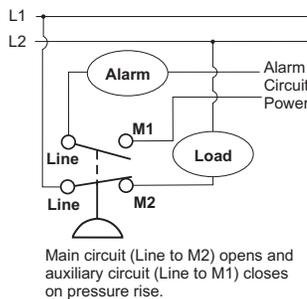
**Typical Wiring for 4-wire 2-circuit Switch used for a
