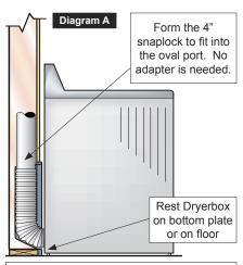
Install box as low as possible and as near to the center of the proposed dryer
