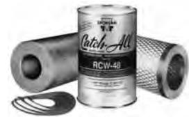
**RC-4864-HH** – Activated Charcoal Core – Order as separate item – Fits types C-480 thru C-19200 Series shells and Replaceable Suction Filter (RSF) shells. This core should be used for wax removal on low temperature systems, and for clean-up of systems that have had a hermetic motor burnout.
