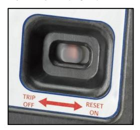
The Sentronic 3 module features a light emitting diode (LED) to provide a visual indication of the oil pressure condition. To aid in troubleshooting, the cover label has a summary of the LED fault indications. Below explains the information provided by the LED.
