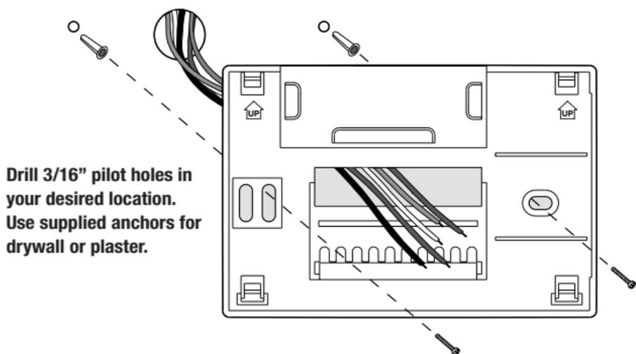
**NOTE:** After sub-base installation, you may insert the quick reference card into the slot on the top of the base.
