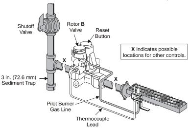
Figure 2: Typical Installation of an H15 Valve with Internal Pilot Gas Flow and Rotor "B" Valve (Models H15\_H)
