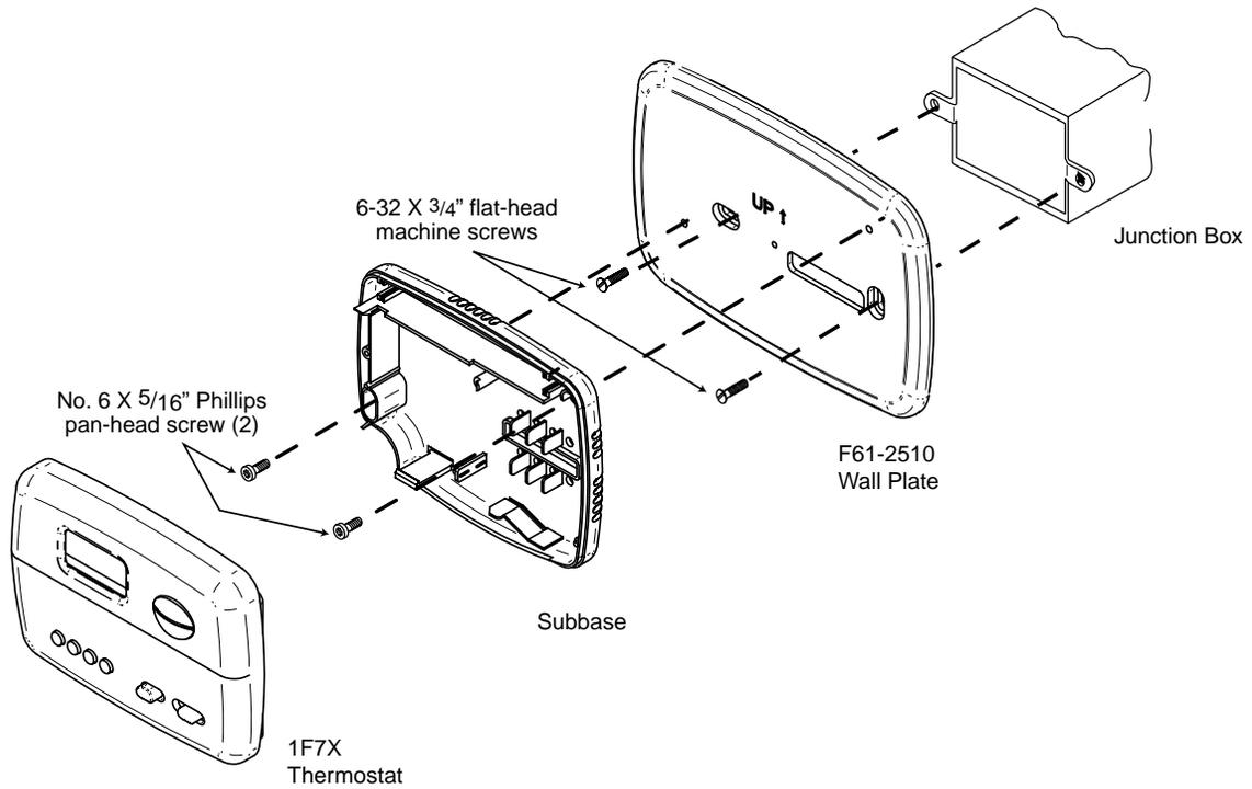
Figure 1. Mounting 1F7X digital thermostat to horizontal junction box.
