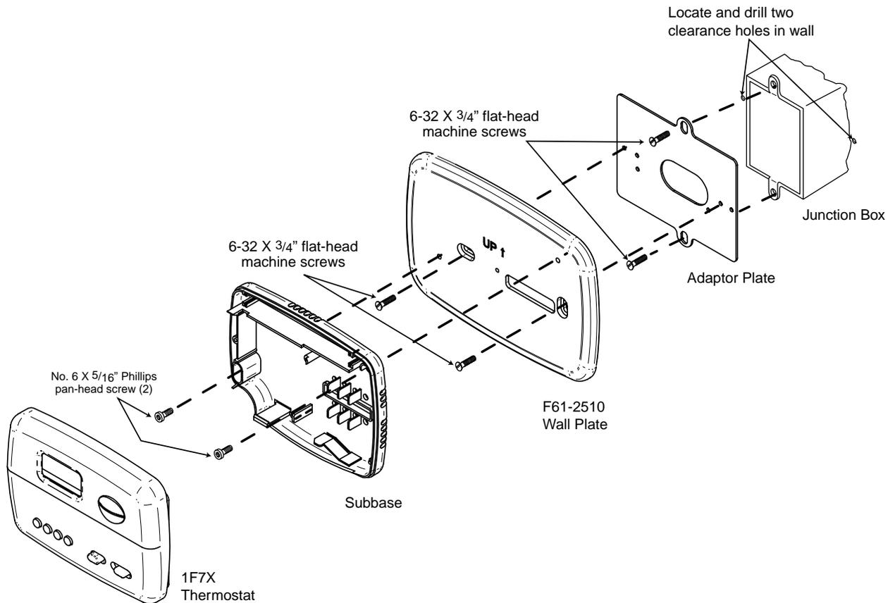
Figure 2. Mounting 1F7X digital thermostat to vertical junction box.
