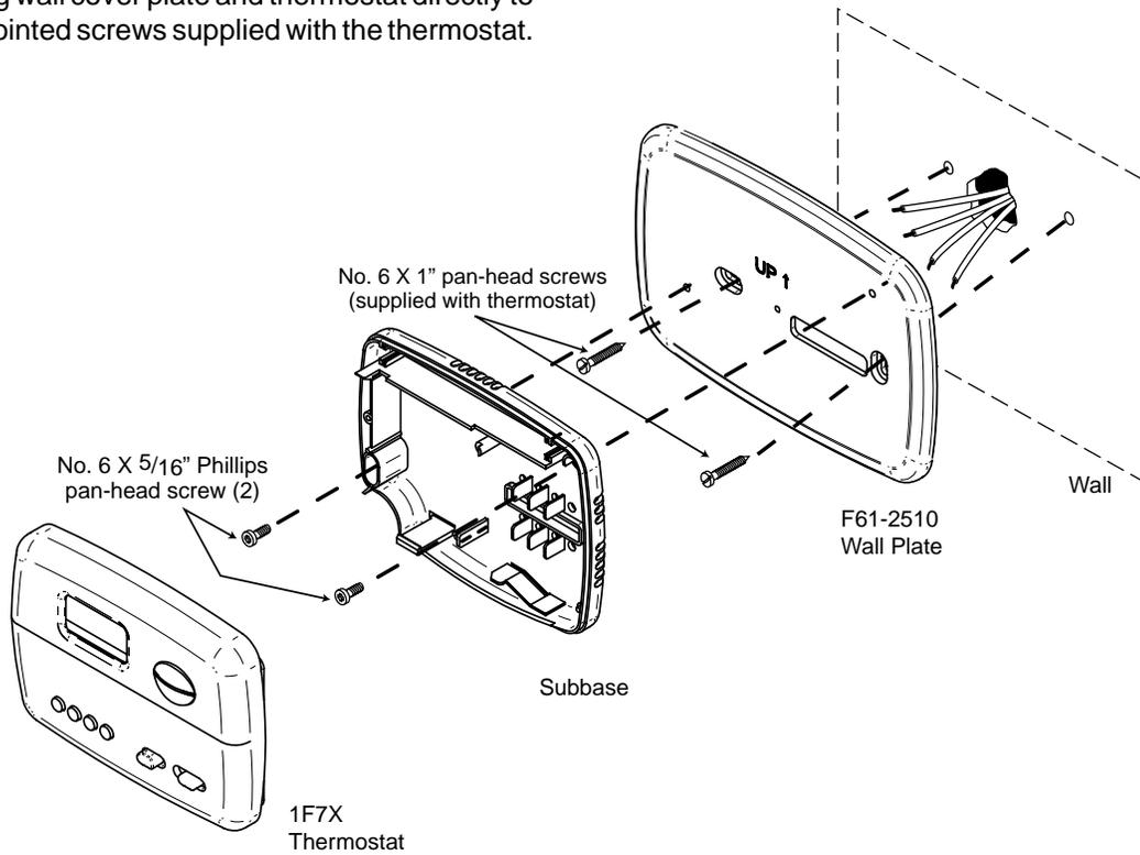
Figure 3. Mounting 1F7X digital thermostat to wall.
