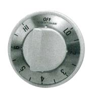
The Model INF control contains a bimetal which regulates the running cycles. This bimetal has a resistance wire wrapped around it which is connected in parallel with the heating unit being controlled and is cycled in unison with the heating element. When the dial is turned to any On position, the cam follower moves out and allows the cycling contacts to close. This completes a circuit through the heating unit
