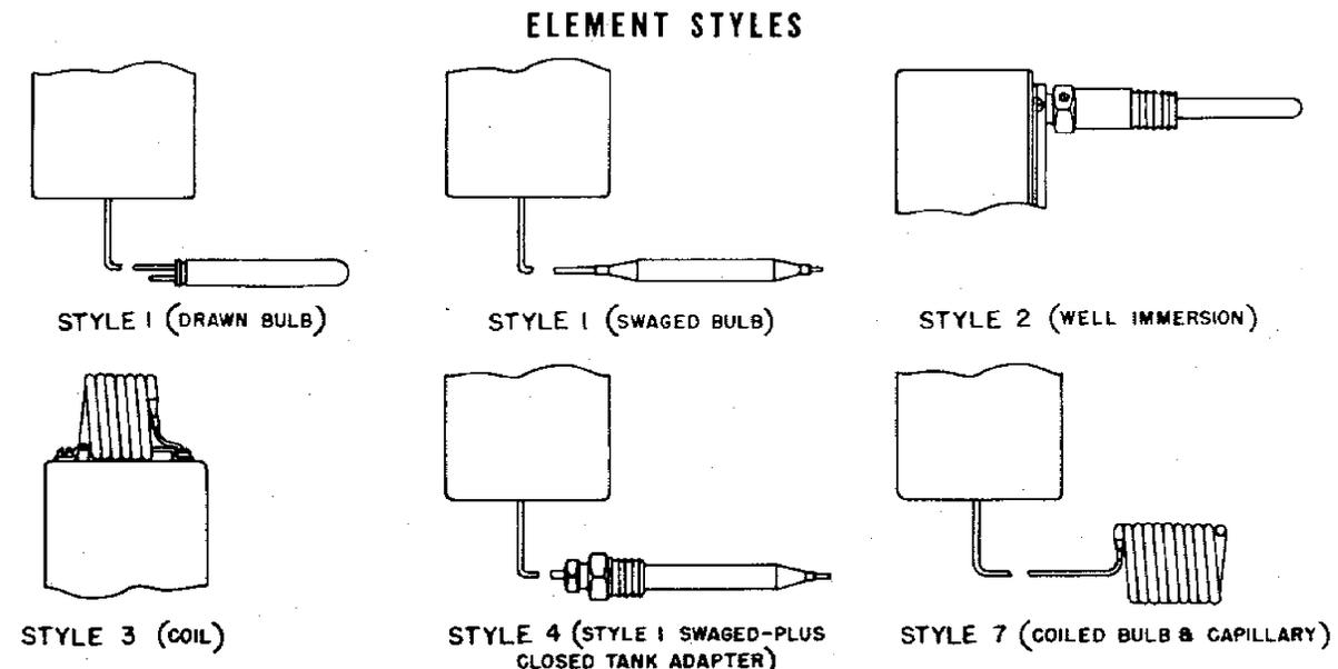
Fig. 3: Element Styles available on Series A19
