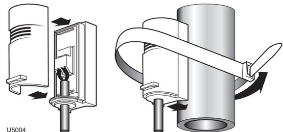
2. Use a system temperature sensor to regulate temperature in the system main piping. (Locate the supply sensor at least six pipe diameters, but no further than 3 feet, downstream from the boiler connection to the main to ensure adequate mixing.)
