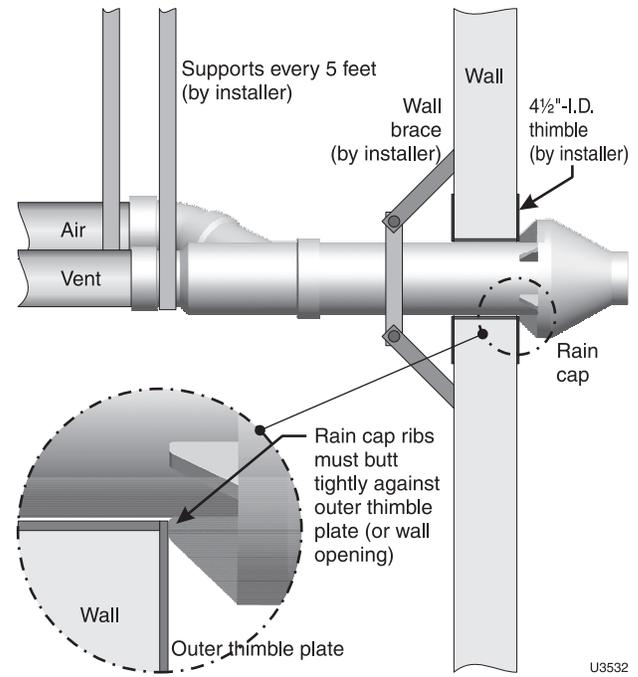
**WARNING** Ensure that the wall material is strong enough to prevent the rain cap from being pushed inward if struck or pushed from the outside.
