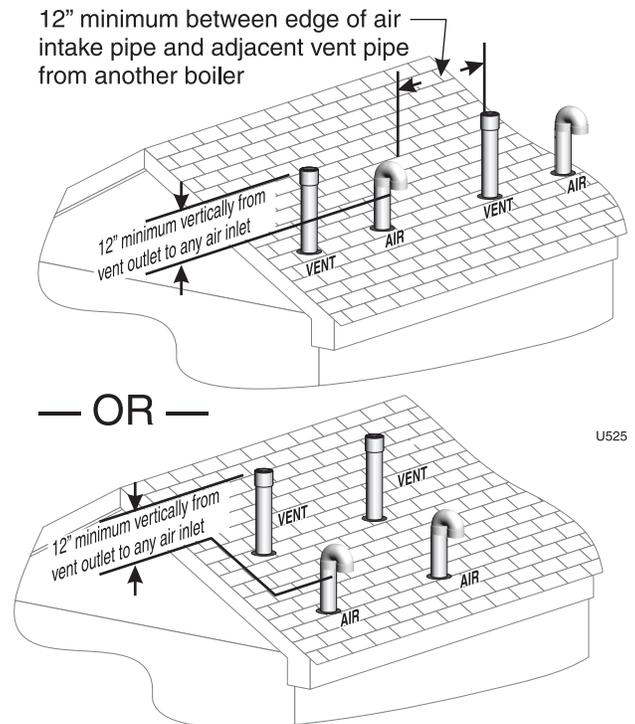
3. The vent piping must terminate in an up-turned coupling as shown in Figure 63, page 46. The top of the coupling must be at least 1 foot above the air intake. The air inlet pipe and vent pipe can be located in any desired position on the roof, but must always be no further than 2 feet apart and with the vent termination at least 1 foot above the air intake.
