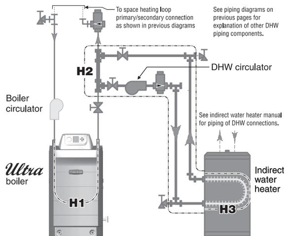
H1 = 0 (no DHW flow through boiler)      H3 = Head loss through water heater
