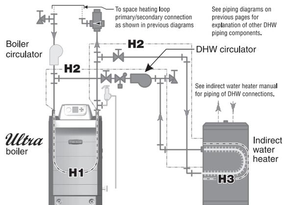
H1 = Head loss through boiler      H3 = Head loss through water heater
