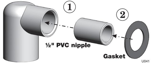
Figure 69 Condensate drain — Ultra-80 & -105
