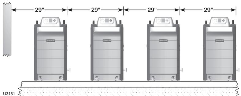
**Figure 3** Back-to-back installation of multiple Ultra boilers
