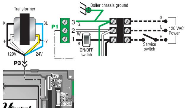
1. Provide and install a fused disconnect or service switch (15-ampere rated recommended) as required by applicable codes.
