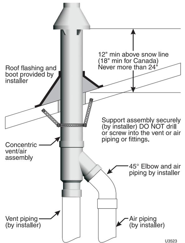
**Figure 61** Alternate piping configuration, using (3) 45-degree elbows to obtain closer pipe centers
