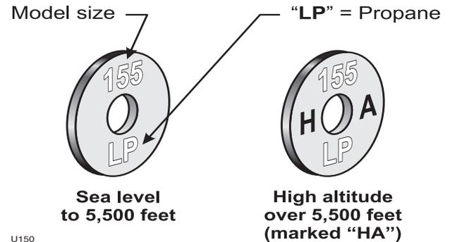
**Figure 6** Installing propane orifice (Ultra-105 or Ultra-80LP ONLY)
