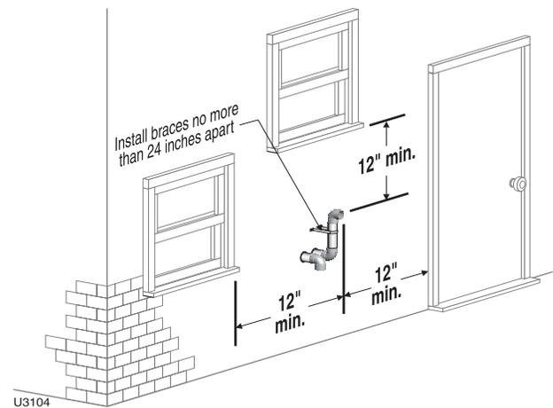
**Figure 51** Sidewall termination with separate pipes — clearances to public walkway or forced air intake
