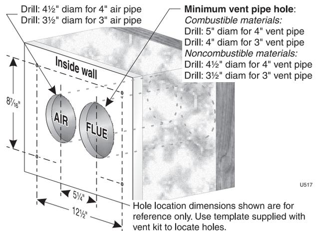
**Figure 41** Termination assembly — Weil-McLain vent/air plate
