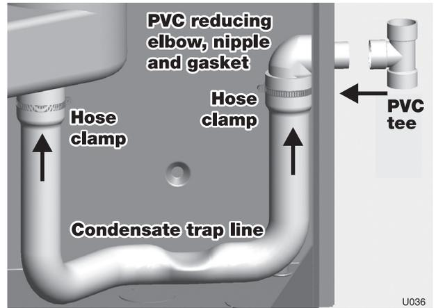
**Figure 72** Condensate drain — Ultra-310
