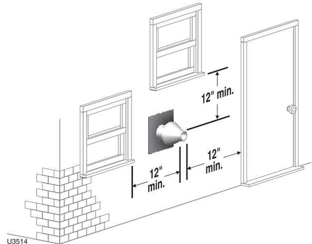
**Figure 45** Termination location — Weil-McLain vent/air plate — clearances to public walkway or forced air intake
