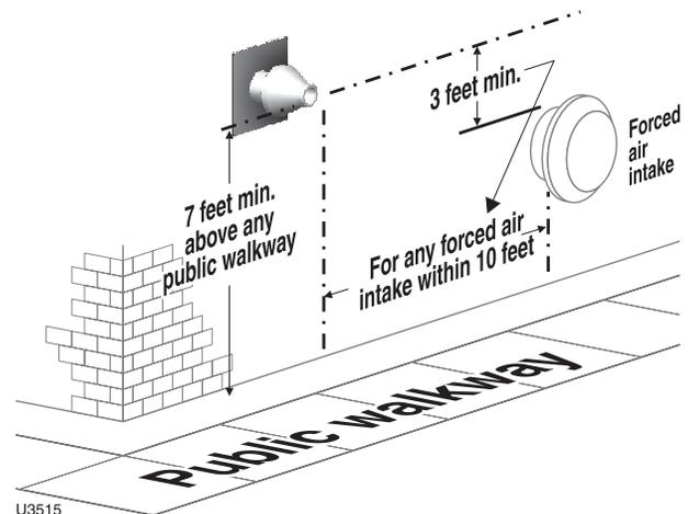
**Figure 46** Termination location — Weil-McLain vent/air plate — multiple boilers — clearance from vent of one to air intake of the next
