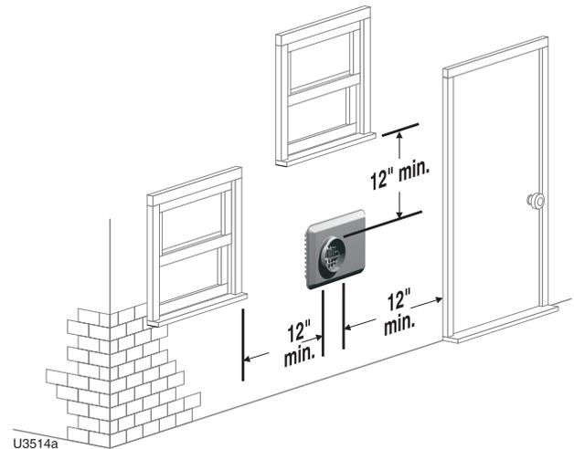
**Figure 38** Termination location — Weil-McLain vent/air plate — clearances to public walkway or forced air intake
