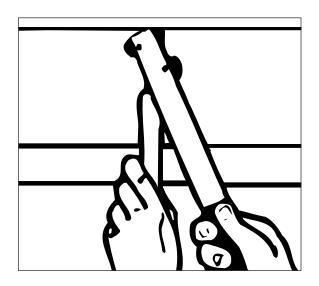
Lightweight aluminum body features an **offset handle** to eliminate knuckle contact with work. Additional spacing holes allows wheels to be adjusted to span greater distances.
