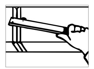
Grasp adjoining duct flanges with wheels of Duct Stretcher to **pull sections together while installing drive cleat** with free hand.
