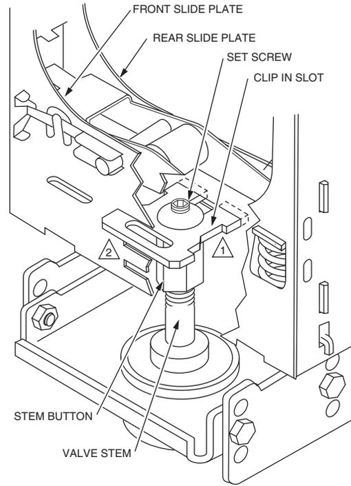
1 CLIP MUST ENGAGE SLOTS ON STEM BUTTON AND REAR SLIDE PLATE.
