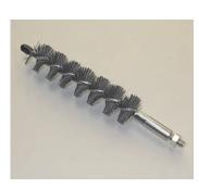
Single stem construction with silicone carbide impregnated nylon. This brush is made with a tapered trim to allow better cleaning of enhanced condenser tubes. The long bristles are designed oversized with the intention of bending over, allowing the aggressive filament to come into maximum contact with the lands. The short bristles are able to get into the grooves. These brushes provide better cleaning and longer life than conventional condenser cleaning brushes.
