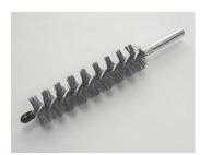
Single stem construction with silicone carbide impregnated nylon recommended for brass tubes. This brush is made oversized so the filament will lav over. resulting in increased contact with surface, providing better cleaning and longer life than conventional condenser cleaning brushes.
