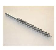
Single spiral/double stem construction recommended for stainless steel tubes. 1/4" and 5/16" dia. brushes with female couplings have 8-32 threads, while 3/8" thru 1" dia. have 12-24 threads. 1/4", 5/16", and 3/8" dia. brushes with male couplings have 8-32 threads, while 7/16" thru 1" dia. have 1/4-28 threads.
