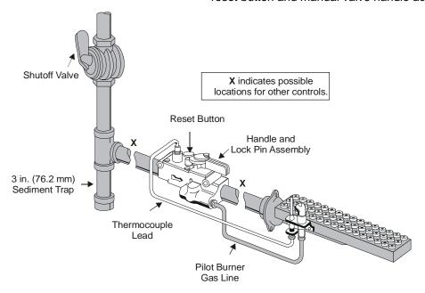
Figure 2: Typical H43 Installation
