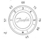
The user can easily set room temperature by turning the dial clockwise or counterclockwise. The diagram to the right shows the appropriate relationship between dial scale numbers and room temperature.
