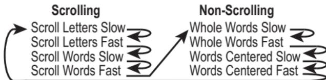
Press the **SETUP** button, then press **MODE** repeatedly until the Scrolling Method setup step appears. Use the **WARMER** or **COOLER** buttons to make selection. Press **MODE** to advance to the next step. Press **SETUP** to leave the setup screens.
