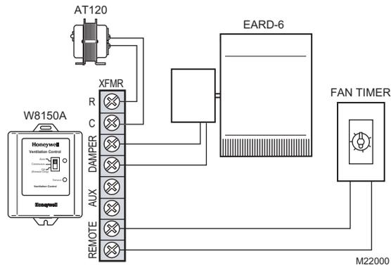
Fig. 7. Using a remote switch or timer.
