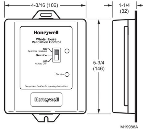
W8150A Ventilation Control dimensions in in. (mm).
