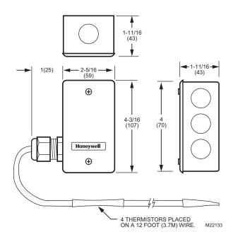
Fig. 9. C7031J, C7041J dimensions in in. (mm).
