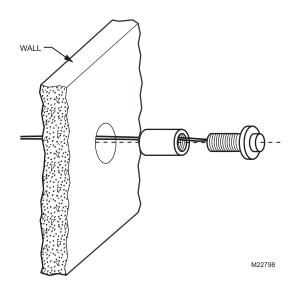
Fig. 18. Mounting sensor in wall with spacer only.
