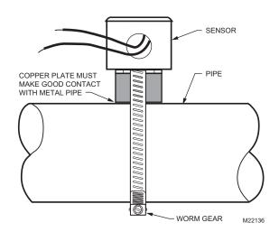
Fig. 15. Strap-on mounting of C7041K Sensor.
