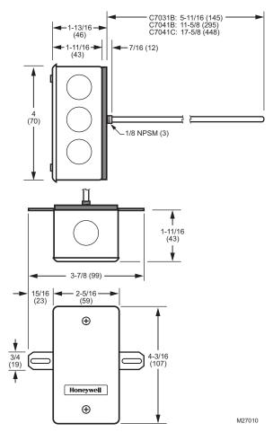
**Fig. 1. C7041B,C dimensions in in. (mm).** NOTE: The C7041D uses the 50001774-001 Well Assembly. See Fig. 5 for dimensions
