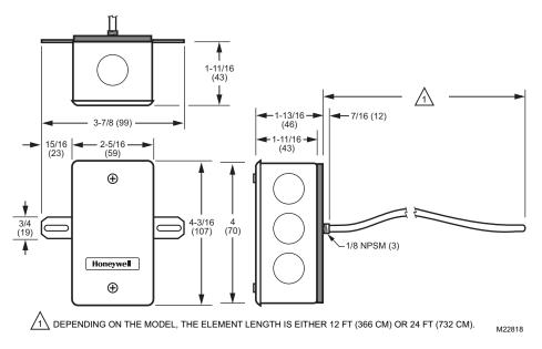
Fig. 7. C7041R dimensions in in. (mm).
