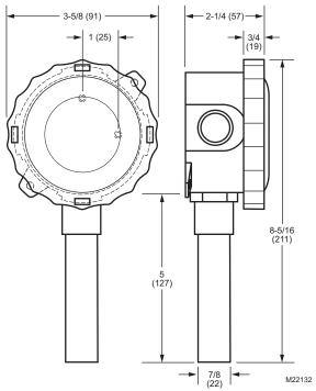
Fig. 5. C7031G, C7041F dimensions in in. (mm).
