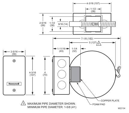
Fig. 8. C7041K dimensions in in. (mm).
