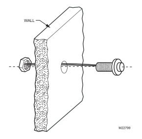
Fig. 17. Mounting sensor in wall with nut only.
