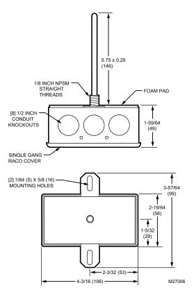
Fig. 4. C7031B dimensions in in. (mm)
