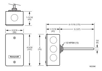
Fig. 6. C7031D, C7041D dimensions in in. (mm)
