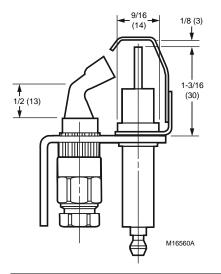
Leadwire Temperature Ratings: (Max. at electrode tip: 968 C)
