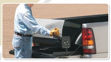
Makes bends to 135 degrees in galvanized sheet steel up to 22 gauge (0.86 mm). A beefed-up 5/16 in. (7.9 mm) plate steel apron and 48 in. (1.2 m) metal width capacity makes the Mini Brake ideal for fabricating plenums or large transitions at the job site.
