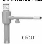
Crankcase Pressure Regulating Valves are designed to prevent overloading of the compressor motor by limiting the crankcase pressure to a predetermined maximum value during and after a defrost cycle or a normal shutdown period. These valves automatically throttle the vapor flow from the evaporator until the compressor can handle the load.
