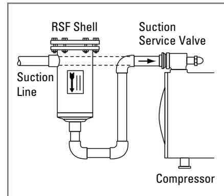
Any pressure loss in the suction line also reduces system capacity significantly. When an RSF shell or replaceable core type Catch-All is used, it is recommended that the cores be removed and filter elements installed when the clean-up job is complete. Obtaining a low pressure drop is particularly important for energy savings on supermarket refrigeration systems. Therefore, suction line filter-driers should be sized generously on these systems.
