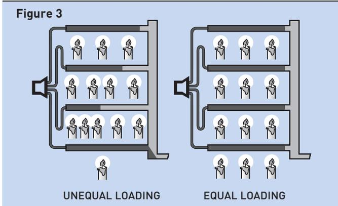
Optimum distributor performance is obtained when the distributor is mounted directly to the TEV outlet. If the distributor cannot be mounted directly to the valve outlet, it can be connected by a piece of **straight** tubing or pipe. The tubing or pipe should not exceed **two** feet, and it should be sized to maintain high refrigerant velocities. Elbows located between the TEV and distributor hinder proper distribution, and are **not** recommended.
