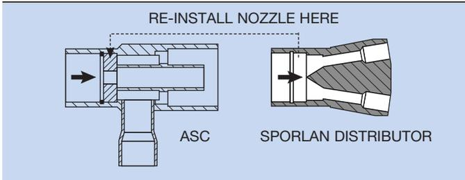
As with side connection type Sporlan distributors, the ASC allows hot gas or liquid refrigerant in the reverse cycle to bypass the nozzle. In addition, the two-phase refrigerant flowing from the TEV passes through the nozzle, and a nozzle tube extension, which terminates at the distributor's
