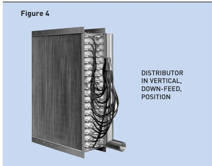
When a system uses two or more distributors, each distributor must be fed by its own TEV. If one valve feeds two distributors, the refrigerant flow will not be divided evenly into the distributors.
