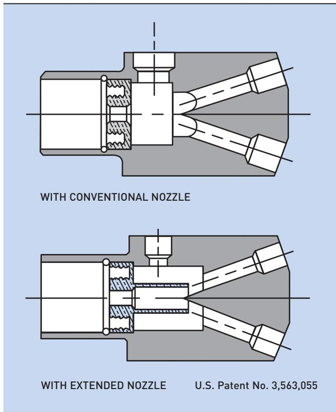
To distinguish side connection distributors with the extended type nozzles from the conventional distributors, the letter "R" is stamped after the designation on the body. For example, the Type **1653R** distributor employs the extended type nozzle. The extended nozzles are also similarly marked: the **GR** nozzle is the extended nozzle used in the Type **1653R** distributor.
