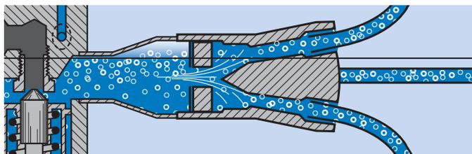
1. Velocity of refrigerant LIQUID-VAPOR MIXTURE increased by flow through nozzle orifice
