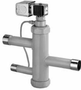
energized the piston and seat assembly shifts to close the suction port and open the discharge gas port, to allow hot gas to flow from the discharge header through the valve to the evaporator outlet.
