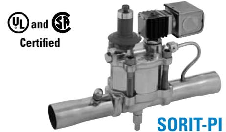
These EPRs are Piloted Internally using the natural pressure drop across the valve to operate and do not require a “high side” pilot connection. Like the (S)ORIT valves, the pilot operated design does not require the “allowable evaporator pressure change” necessary with the direct acting models, and can be simply sized based on design evaporator temperature and available pressure drop across the valve at full load conditions.
