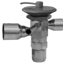
The Type RE valve is a small balanced port valve designed for use on refrigeration applications as well as residential and small commercial air conditioning and heat pump units. The balanced port design provides exceptional control of refrigerant in both directions, making this valve an excellent choice for heat pump systems.
