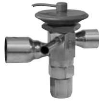
Type RC valves contain internal check valves to allow reverse flow on heat pump applications. This eliminates the need for an external check valve piped around the TEV for reverse flow. The RC valve can be used on Heat Pump and Air Conditioning (cooling only) applications.
