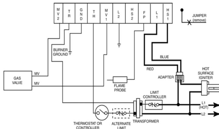
**YELLOW FLASHING INDICATOR (IMPROPER POLARITY LOCKOUT):** Yellow indicator will flash if the polarity is not correct as diagrammed above on both the primary and secondary of the system transformer.
