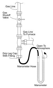
17. Connect a calibrated water manometer (or appropriate gas pressure gauge) at either the gas valve inlet pressure boss or the gas piping drip leg. See gas valve figure for location of inlet pressure boss.
